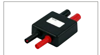
912008000: 10 ohms shunt, 0.1%, 0.15A max
