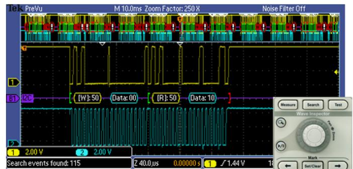
Search - I<sup>2</sup>C decode showing results from a Wave Inspector search for Address value 50. Wave Inspector controls provide unprecedented efficiency in viewing and navigating waveform data.
